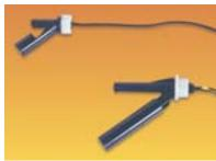
**Compact 151-643** L=73 (overall), 60 (actuator), Mtg. hole dia=12.7 151-644 L=70 (overall), 57 (actuator), Mtg. hole dia=16.5 732-709/607-320 L=88 (overall) 55 (actuator), Mtg. hole dia=16.5 Max. vessel wall thickness=4
